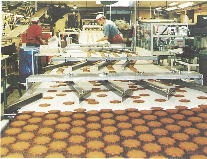
More than 1,600 tons of gingerbread cookies annually are produced by Annas Pepparkakor on continuous steel belts from Sandvik Process Systems.
