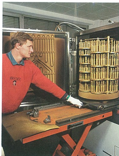
Titanium-nitride coating of Titex drills in Frankfurt, Germany.
