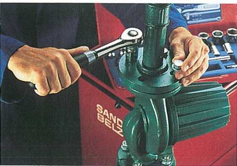
A new ergonomically designed handle featuring a socket ratchet with one-hand-use facility was introduced during 1995.
