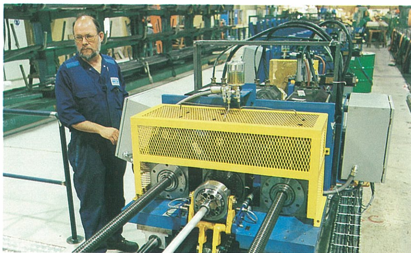
A new pilger mill from Sandvik Special Metals (of the type for which the Haglund Medal was awarded in 1990) increases capacity by 70% in Tube Mill 87 in Sandviken.
