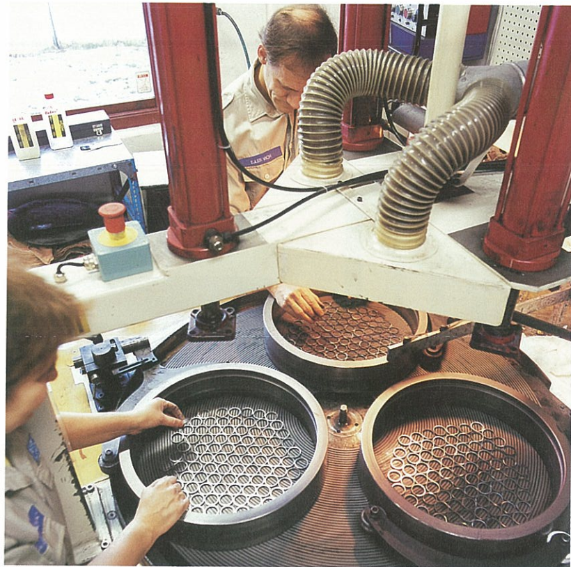
Seal rings for submersible pumps are manufactured at Sandvik Hard Materials' plant in Denmark.
