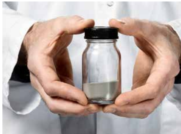
The super-duplex metal powder is produced and optimized for 3D printing.
