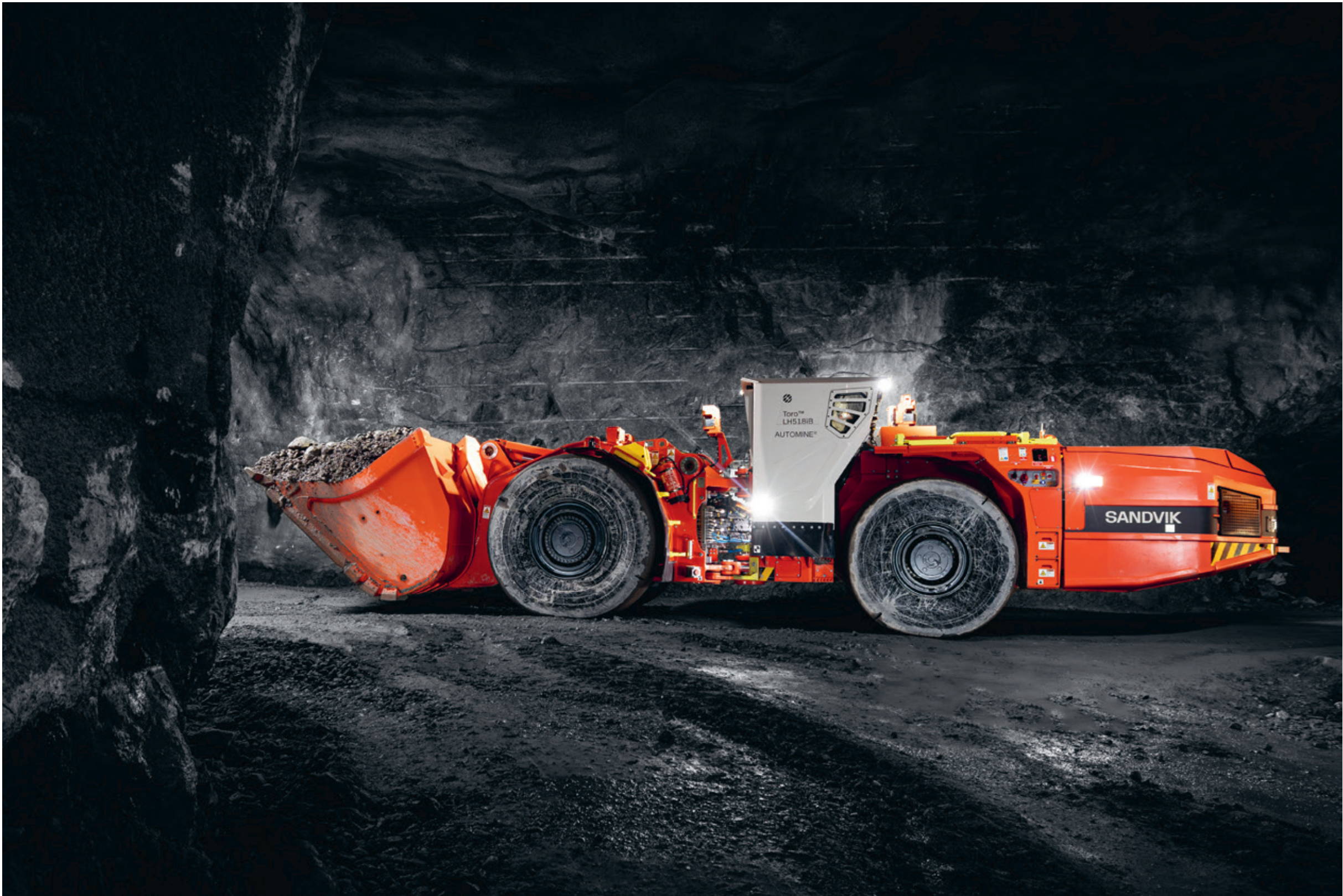
Battery-electric loaders from Sandvik have zero underground diesel emissions.
