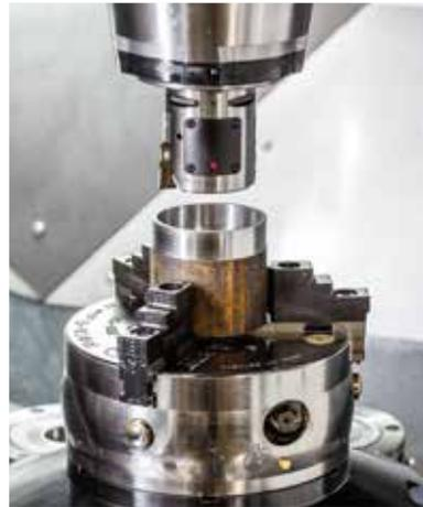
CoroPlus® is a new platform of connected tools and software, essentially comprising technologies that can send and receive data. The system gives insights into the machining environment that can be used to plan and optimize production.
