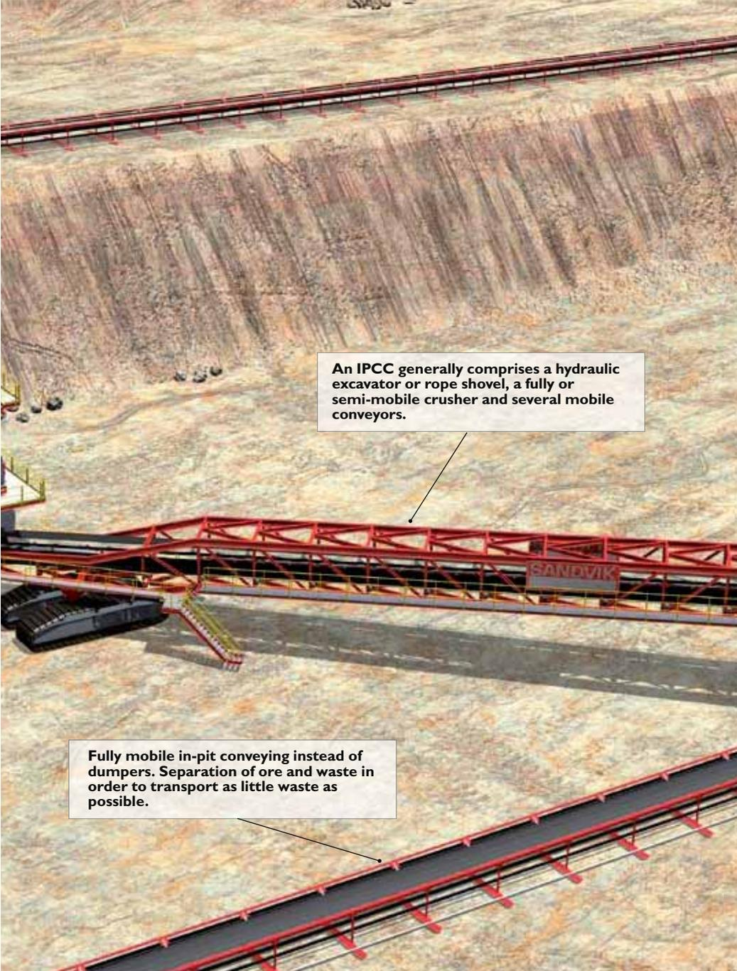
An IPCC generally comprises a hydraulic excavator or rope shovel, a fully or semi-mobile crusher and several mobile conveyors.
