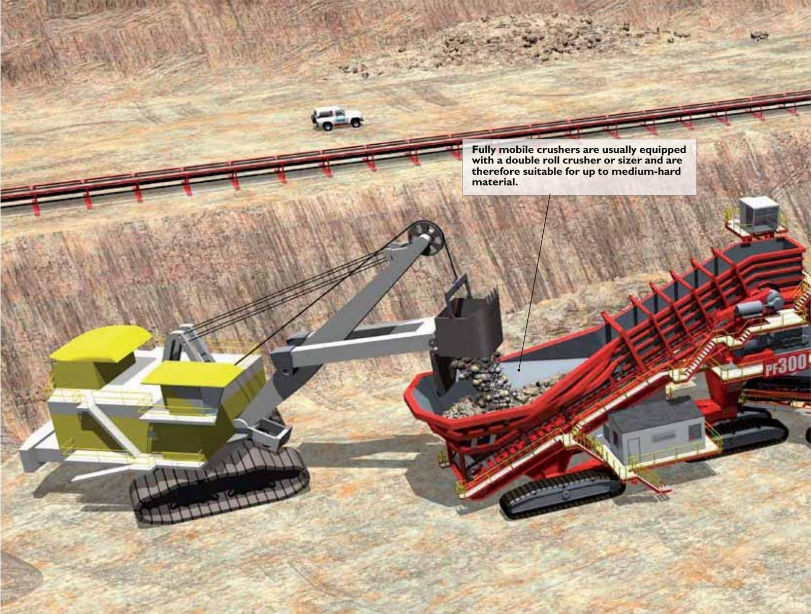
Fully mobile crushers are usually equipped with a double roll crusher or sizer and are therefore suitable for up to medium-hard material.
