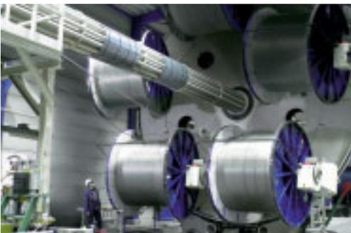
Sandvik's seamless, stainless-steel tubes on coils play a key role in production of umbilicals for the oil/gas industry
