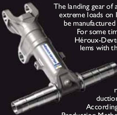
The landing gear of an aircraft is exposed to extreme loads on landing. It must therefore be manufactured from a tough material.
