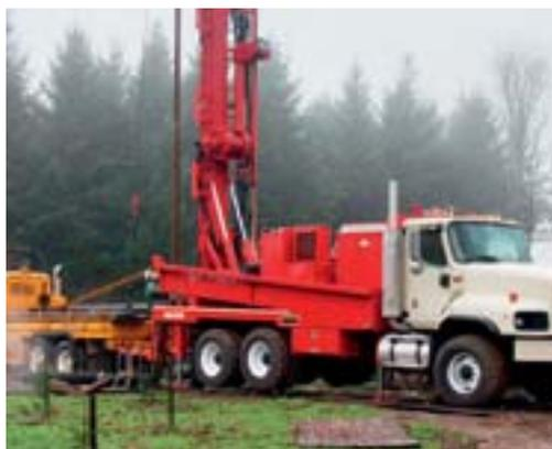
Subterranean heat involves drilling a hole in the bed-rock to extract heat from the groundwater. One of Sandvik's production units was able to reduce electricity consumption substantially using this method.
