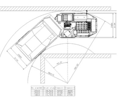
Sandvik's newly launched trucks for mining feature many new innovative solutions, such as a small turning radius.
