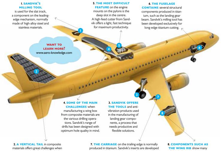
2. A VERTICAL TAIL in composite materials offers great challenges when it comes to edging. Sandvik's endmill in PCD (vein and brazed) and diamond-coated cutters can be engineered to suit this application.
