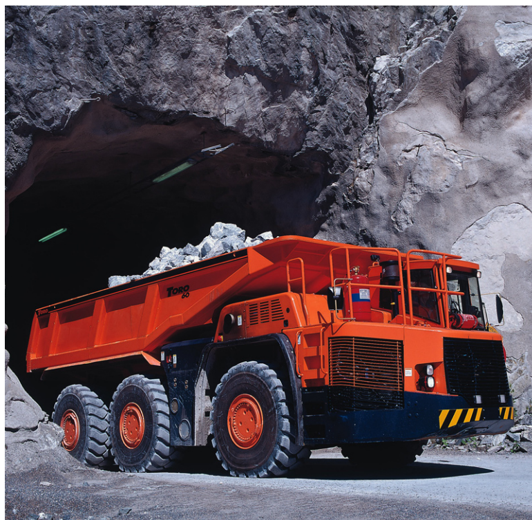
Sandvik Mining and Construction's total offering to customers continues to develop. The Toro 60 underground, with steel frame and three axles, is an example of a new philosophy – powerful but agile and fast dump trucks.
