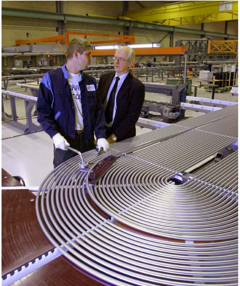
Peter Gossas, President of Sandvik Materials Technology, during one of many visits to production facilities. Photo shows the final assembly of steam generator tubes at the Tube Plant 68.
