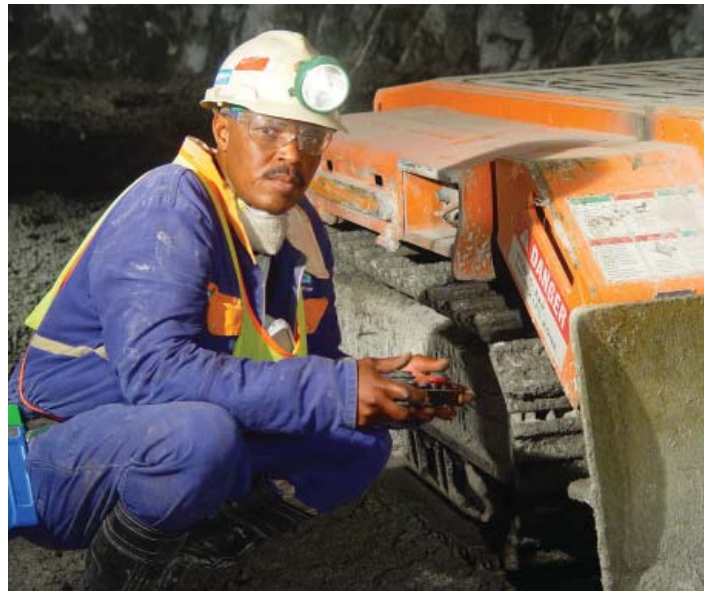
One of Sandvik Mining and Construction's service operators in South Africa with a very low loader, specially designed for the narrow stopes of platinum mines.
